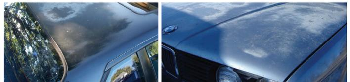
Sun damage typically affects large body surfaces like hoods and roofs. When you see small patches of peeling clear-coat, especially in corners and other hard-to-reach areas, they may indicate a poorly prepped paint job.
